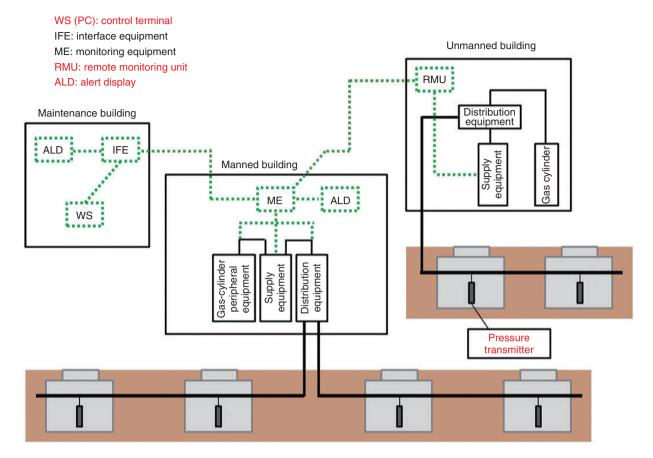
Fig. 3. Configuration of gas facilities.
