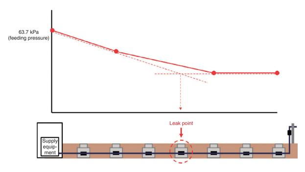
Fig. 5. Inference of gas leak point.
