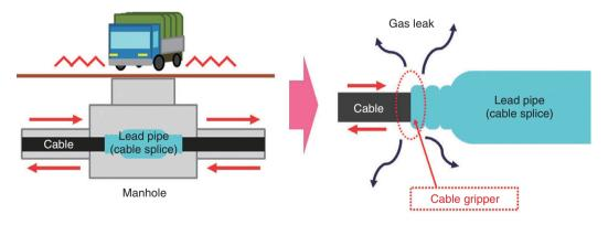
Fig. 2. Gas leak caused by cable movement.
