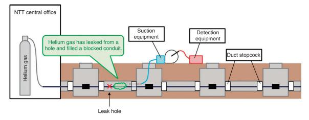
Fig. 7. Gas leak search using helium gas.
