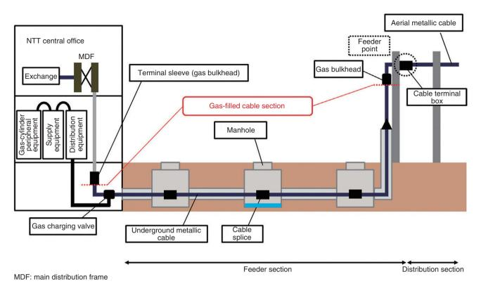
Fig. 1. Configuration of metallic facilities.
