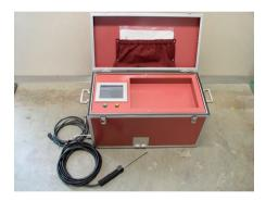
Fig. 8. Helium gas detection equipment.
