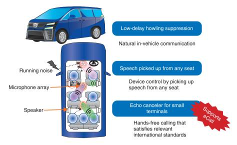
Fig. 4. Intelligent microphone for cars.
