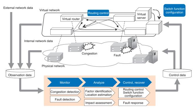
Fig. 1. Proactive controlled network [1].
