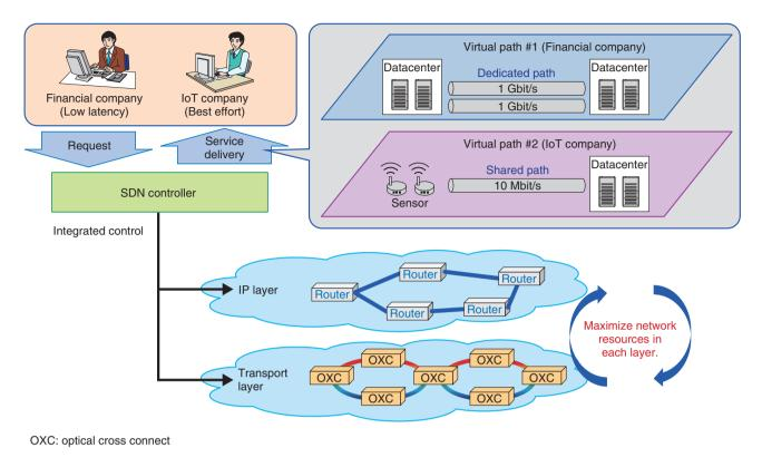
Fig. 4. Multi-layer SDN control technology.
