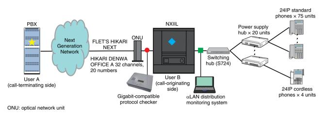
Fig. 1. Connection configuration and data collection points.
