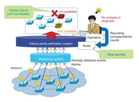
Fig. 4. Automatic failure points estimation system.
