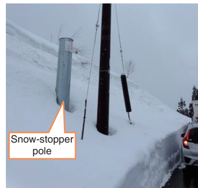
Fig. 6. Trial of snow-stopper poles with in-use utility poles.
