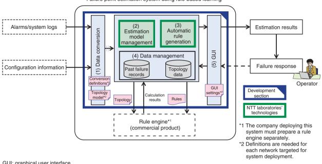
Failure point estimation system using rule-based learning
