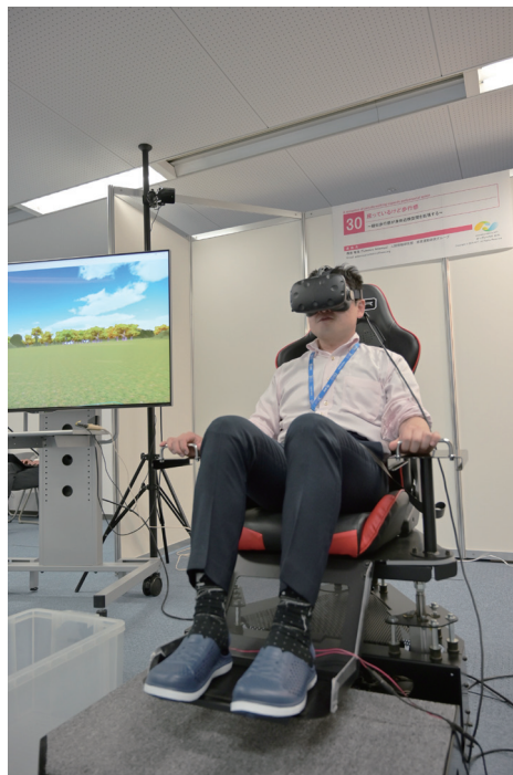
Fig. 5. Pseudo-walking sensation created using a motorized chair and vibration shoes.
