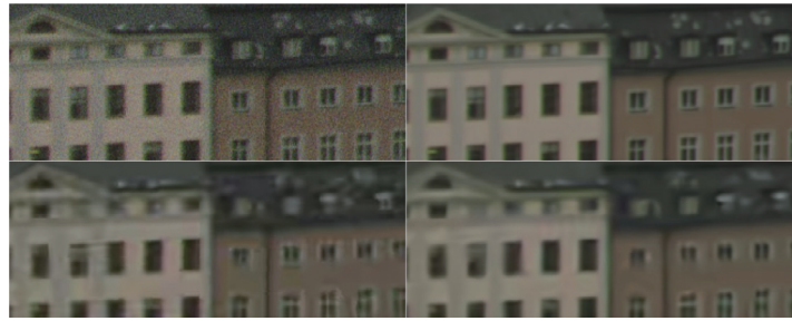
Fig. 8. Rigid-object video-coding results based on real-entity mining approach [13]. (top-left) Former Versatile Video Coding (VVC); experimental model JEM5, rate = 1,857,505 bytes (noisy, similar to original), (top-right) real-entity mining based coding with super-low-rate mode, rate = 13,169 bytes (no noise and crisp), (bottom-left) H.265/HEVC (HM16), rate = 15,061 bytes (distorted), (bottom-right) JEM5, rate = 13,617 bytes (distorted).
