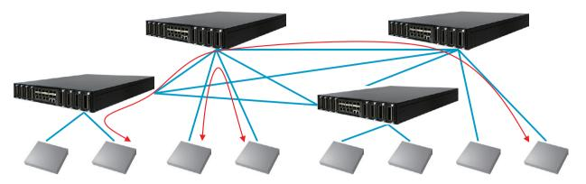
Fig. 1. Full mesh network topology with whitebox packet transponder.
