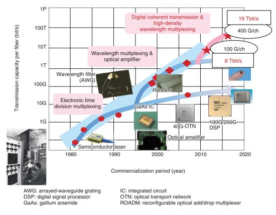
Fig. 2. Progress in photonics technology enabling traffic growth.
