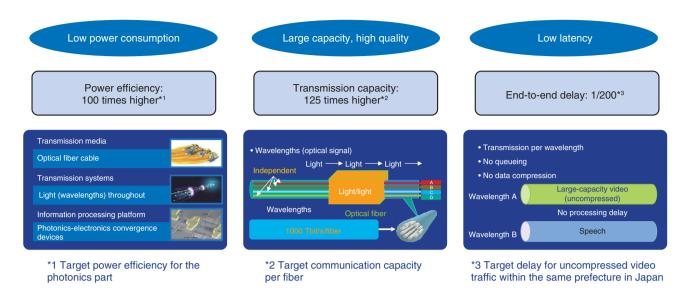
Fig. 1. Target performance of All-Photonics Network.
