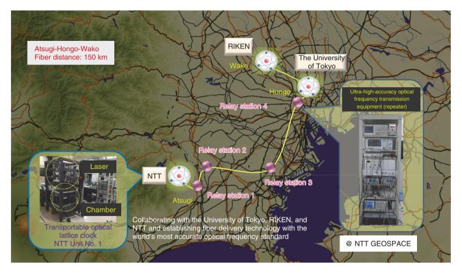
Fig. 6. Optical lattice clock network trial.
