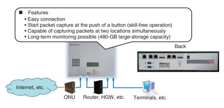
Fig. 4. Packet-capture tool Cap-two (developed by TASC).
