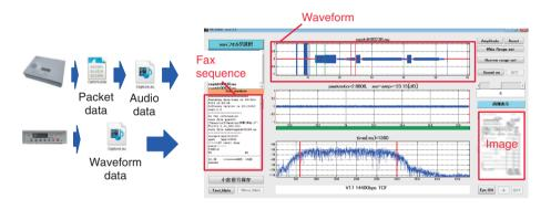
Fig. 6. Facsimile Communication Analyzer (commercial software).
