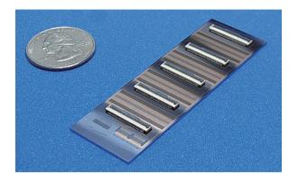
Fig. 3. Photograph of fabricated 16 × 16 MCS.
