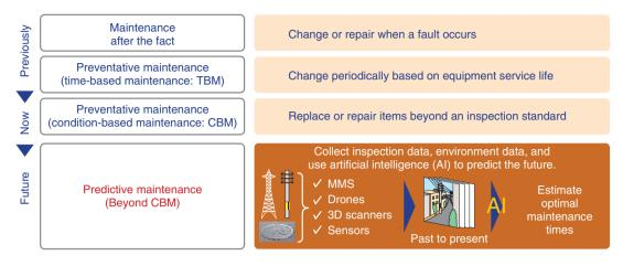
Fig. 8. Utilization for smart maintenance.
