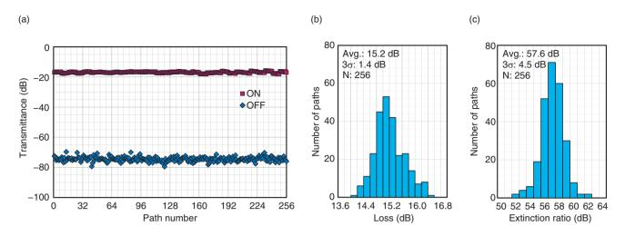
Fig. 5. (a) On-state and off-state transmittance for all 256 paths, and histograms of (b) insertion loss and (c) extinction ratios.
