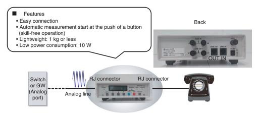
Fig. 5. Analog Logger (developed by TASC).
