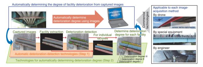
Fig. 4. Determining degree of deterioration with AI.
