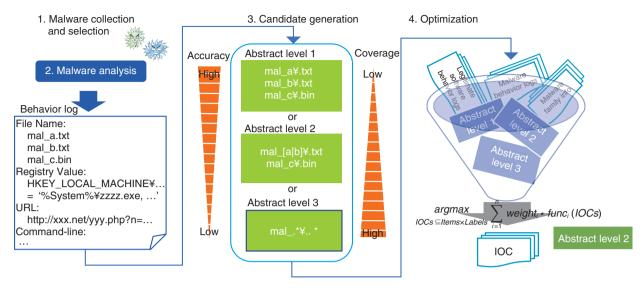
Fig. 1. Automatic generation of IOC.
