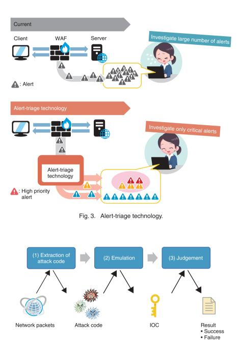
Fig. 4. Basic functions of alert-triage technology.
