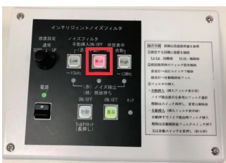
(b) When the built-in EMI filter is applied
