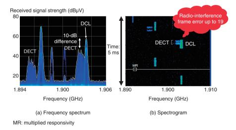
Fig. 4. Results of measuring radio environment.
