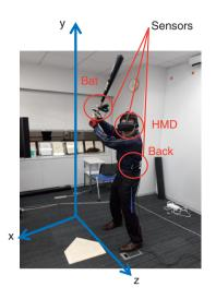
Fig. 3. Swing movement is measured in three directions by using sensors.
