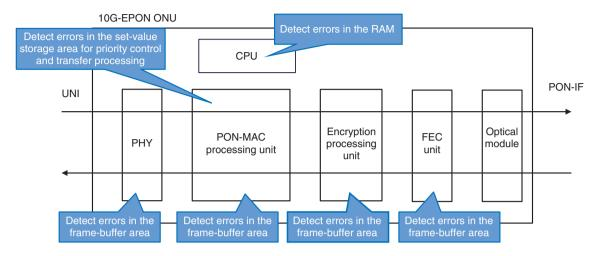
Fig. 4. 10G-EPON ONU functional block and soft error detection.
