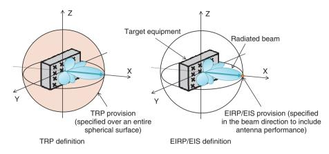
Fig. 1. Definitions used in the RF specification of NR base stations and terminals.
