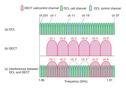
Fig. 1. Frequency allocation of the DCL and DECT.
