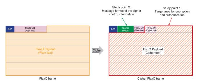
Fig. 5. Example of FlexO frame encryption.
