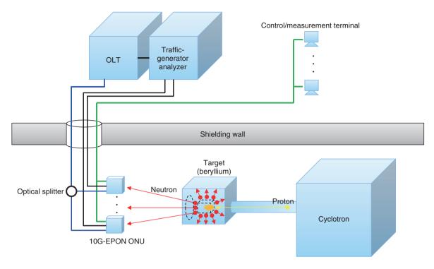
Fig. 6. Neutron irradiation test.
