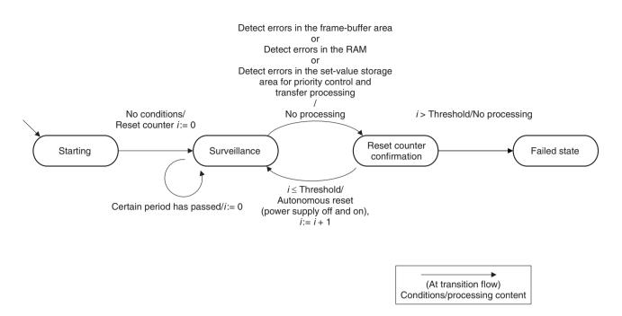
Fig. 5. Transition flow of the autonomous reset function.
