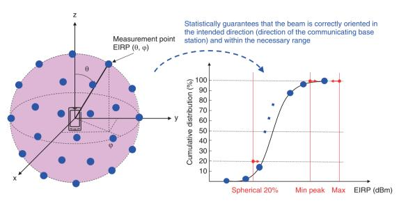
Fig. 2. OTA EIRP evaluation technique using a cumulative distribution.
