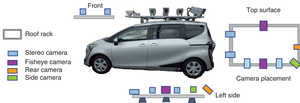
Fig. 2. Our MMS (camera placement).
