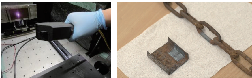
Fig. 7. Example of derusting experiment using our prototype laser-emission head of the rust remover we are developing.
