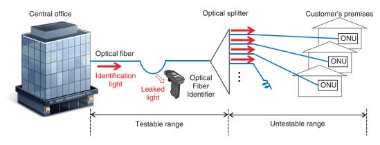
Fig. 1. Fiber identification in optical access networks.
