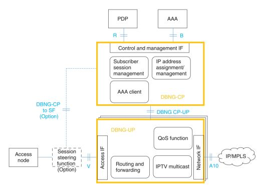
Fig. 2. Newly defined functional blocks and interfaces for the DBNG in TR-459.
