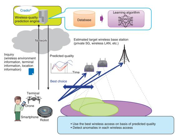
Fig. 4. Prediction - Wireless-network-quality prediction and estimation.
