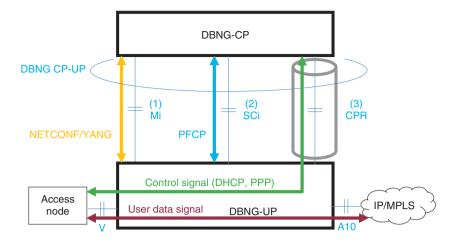
Fig. 3. Conceptual diagram of interfaces between DBNG-CP and DBNG-UP.
