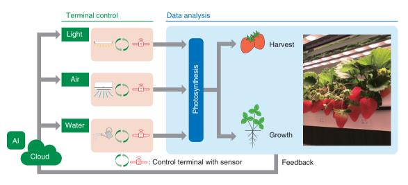
Fig. 3. Cultivation technology used in a strawberry plant factory.
