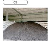
The fermentation/decomposition beds are collected and turned into fully matured compost through secondary and tertiary fermentations at the recycling center, after which, the fully matured compost is recycled as soil conditioner.
