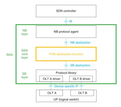
Fig. 4. Conceptual diagram of BAA.
