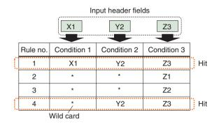
Fig. 3. Concept of NTC using partial match search.
