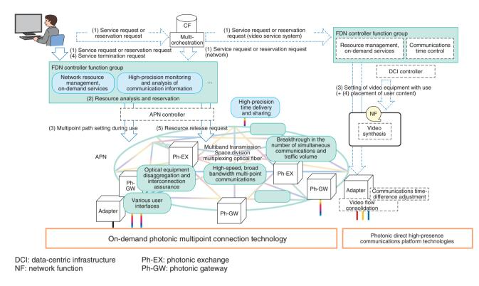
Fig. 3. On-demand photonic multipoint connection technology workflow.
