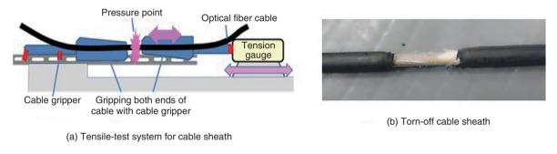
Fig. 7. Tensile test on cable sheath.
