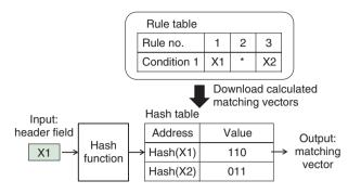
Fig. 6. Operation of hash-based NTC, which obtains a matching vector from the hash table. The matching vector is calculated in advance and downloaded to the hash table.
