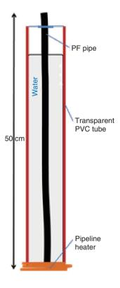
Fig. 4. Lifting pipe simulated with transparent PVC tube.
