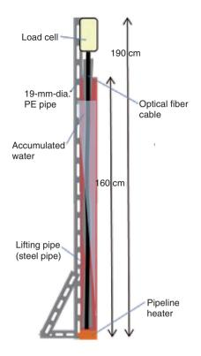
Fig. 3. Apparatus for reproducing lifting pipe.
