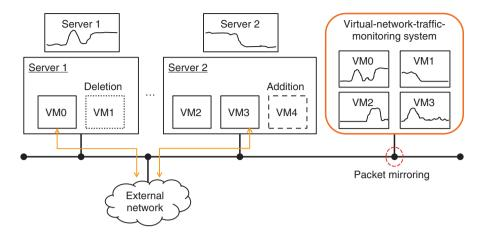
Fig. 1. Network-traffic monitoring using virtual-network-traffic-monitoring system.
