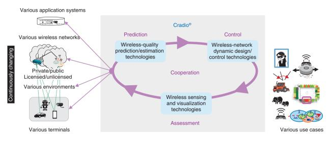
Fig. 2. Multi-radio Proactive Control Technologies (Cradio®).
