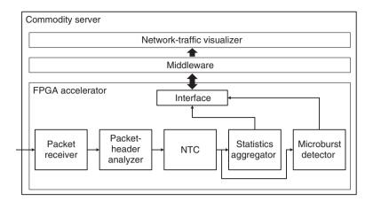
Fig. 2. Block diagram of our virtual-network-traffic-monitoring system with FPGA accelerator.
