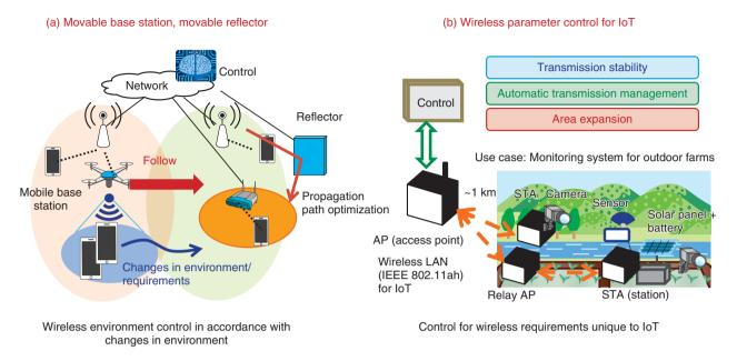
Fig. 5. Wireless-network dynamic design/control technologies.
