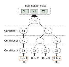
Fig. 4. Network-traffic classification using search tree.
