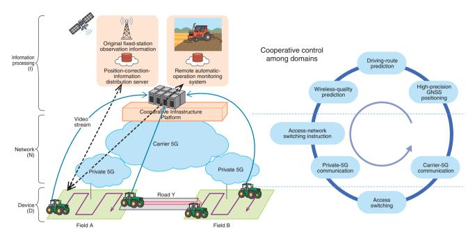
Fig. 5. Cooperative Infrastructure Platform and coordinated operation of information processing, network, and devices.
