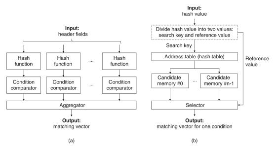
Fig. 7. Block diagrams of hash-based NTC: (a) overall architecture and (b) detailed condition comparator.
