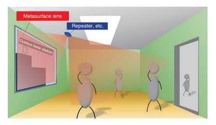
Fig. 6. Example of using a transparent metasurface lens.
