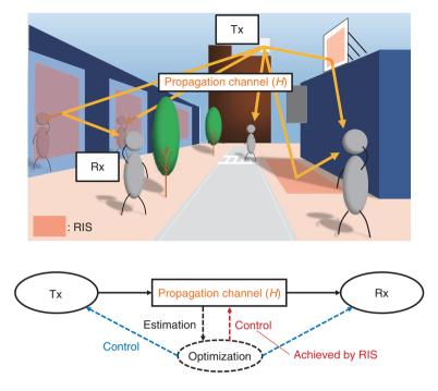
Fig. 1. Conceptual diagram of IRE.
