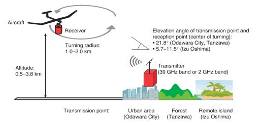
Fig. 6. Illustration of the airborne propagation measurement test.
