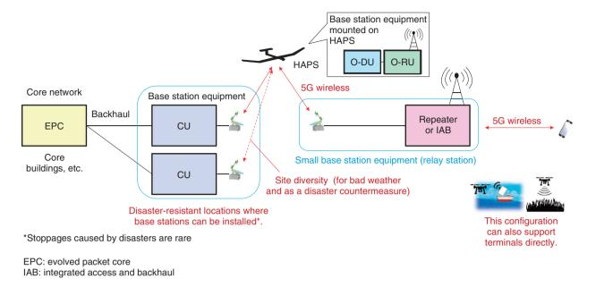
Fig. 5. Example of cooperative configuration when HAPS is used for backhaul.
