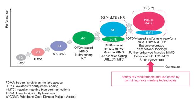
Fig. 3. Technological development of mobile communication systems towards 6G.
