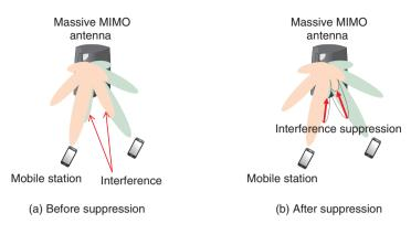
Fig. 1. Conceptual diagram of interference suppression by digital BF.
