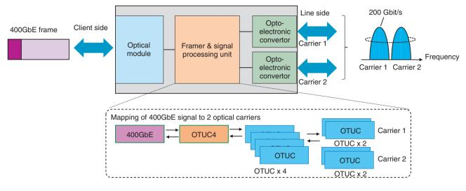
Fig. 4. Multi-carrier transmission of 400GbE signals.
