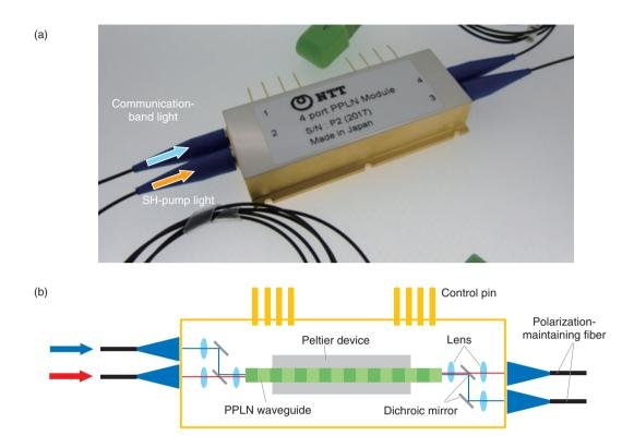
Fig. 2. (a) Overview of fabricated PPLN-waveguide-based OPA module, which has four pigtailed optical fibers as I/O ports.
