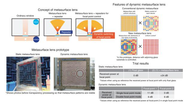
Fig. 5. Concept of making windows into radio-wave lenses by transparent metasurface lens.
