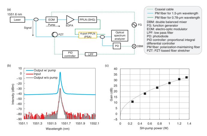
Fig. 3. (a) Experimental setup for degenerate PSA. (b) Measured spectrum of amplified light [18]. (c) External gain of PSA as a function of the input pump power [18].
