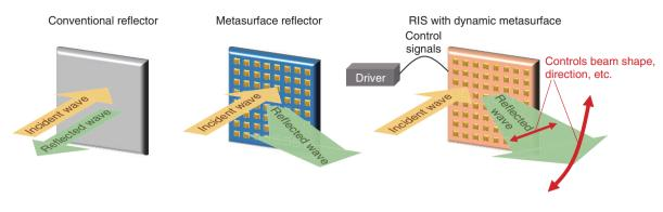
Fig. 3. Conceptual diagram of RIS using metasurface technology.
