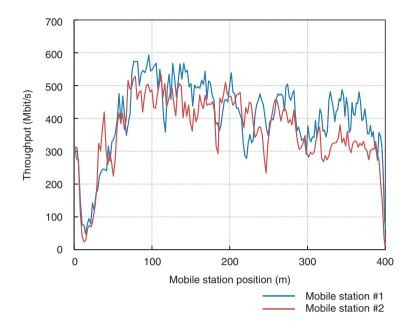
Fig. 6. User throughput for base station switching at 90 km/h.
