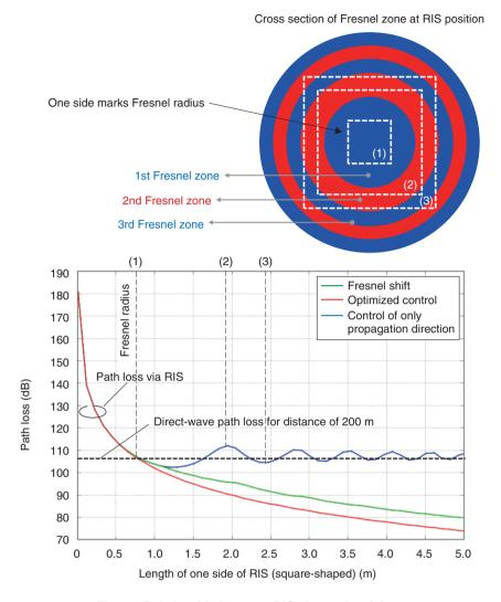
Fig. 2. Relationship between RIS size and path loss.
