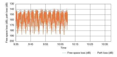
Fig. 8. Propagation loss time series data in the 39 GHz band at Odawara City (line of sight)/2 km turning diameter.
