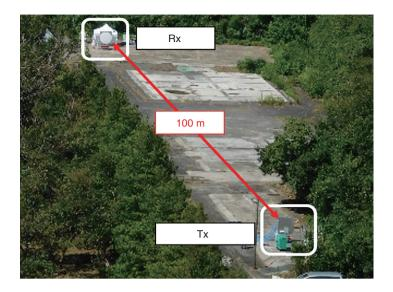
Fig. 7. Experimental environment for wireless OAM multiplexing transmission at a distance of 100 m in the field.
