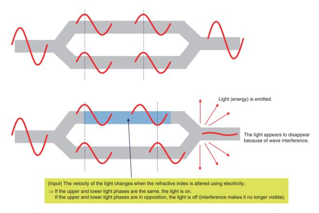
Fig. 1. Principle of Mach-Zehnder electro-optic modulators.
