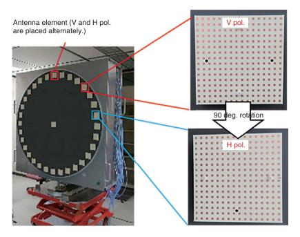
Fig. 5. Prototype of OAM transmission equipment.
