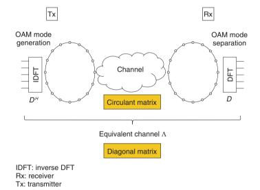
Fig. 4. Schematic of OAM multiplexing system.
