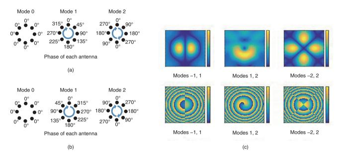
Fig. 3. (a) Generation of OAM modes with a UCA, (b) separation of OAM modes with a UCA, (c) intensity distribution (above) and phase distribution (below) of combined OAM modes (L is the number of OAM modes).
