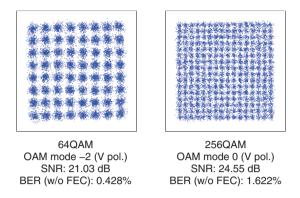
Fig. 9. Representative constellation diagrams of 64 QAM and 256 QAM.
