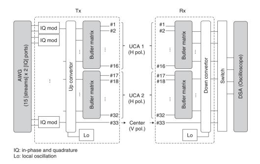
Fig. 6. Block diagram of our experiment.
