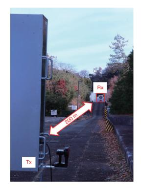
Fig. 8. Experimental environment for wireless OAM multiplexing transmission at a distance of 200 m in the field.
