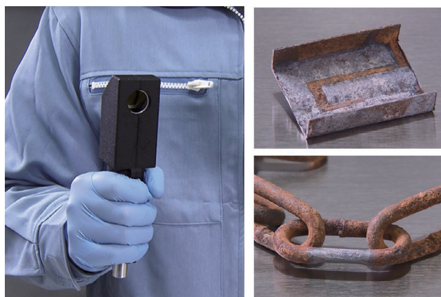
Fig. 1. Prototype rust-removal tool (left) and example of rust removal (right) [1].
