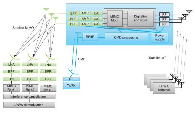
AMP: amplifier BPF: band-pass filter CMD: command signal D/C: down converter
