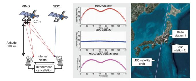
Fig. 4. Capacity enhancement using LEO-MIMO.
