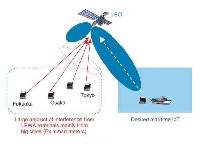
Fig. 2. Satellite blind beamforming.
