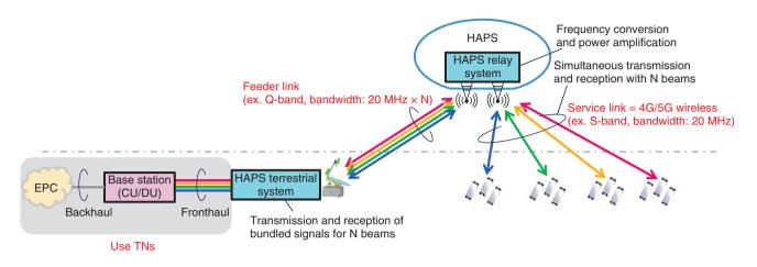
Fig. 3. Example of cooperative configuration when HAPS is used for direct access.
