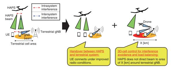
Fig. 4. Handover and 3D-cell control technology.
