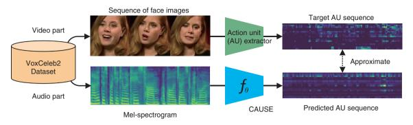
Fig. 2. Training crossmodal action unit sequence estimator (CAUSE).
