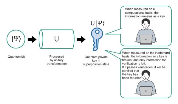
Fig. 2. How a quantum private key works.
