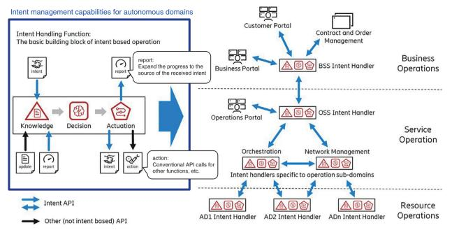
Fig. 4. Autonomous networks and intent.
