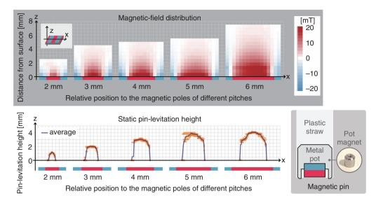
Fig. 3. The spatial magnetic flux density above the different magnetic stripes affects the levitation height of the magnetic pins.
