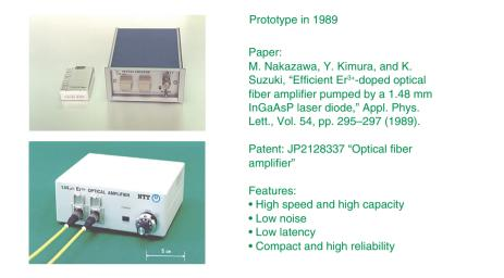
Fig. 1. World's first semiconductor-laser-pumped EDFA.
