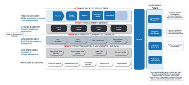
Fig. 5. Closed-loop automation architecture.
