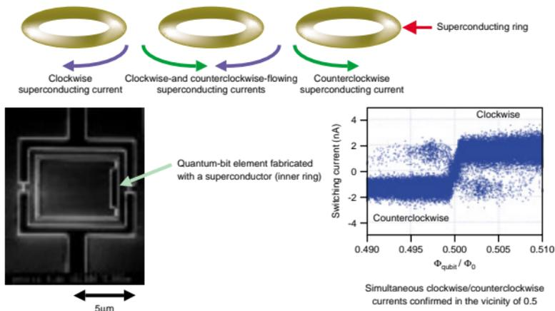
Fig. 2. Quantum-bit elements.
