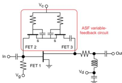
Fig. 8. Circuit configuration of the low-noise variable-gain amplifier.
