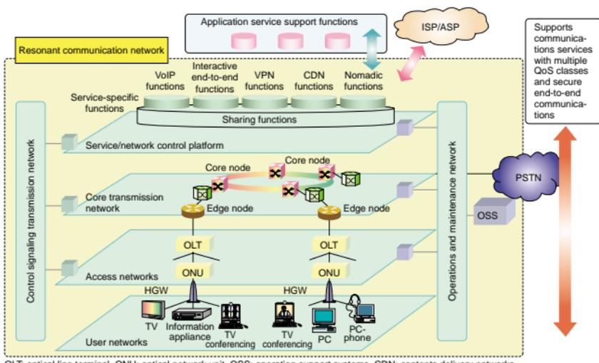
Fig. 2. Resonant communication network architecture.
