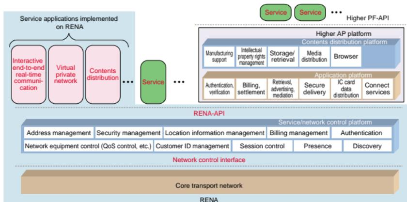
Fig. 5. Configuration of the service/network control platform.
