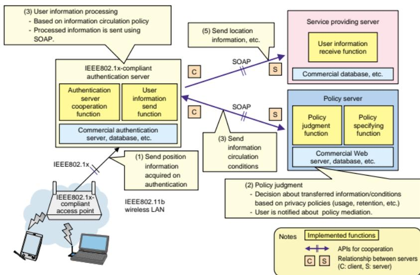
Fig. 7. Architecture of prototype system.
