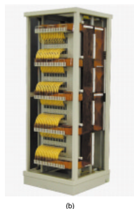
Fig. 6. 128x128 switch subsystem: (a) logical arrangement and (b) photograph of switch subsystem.
