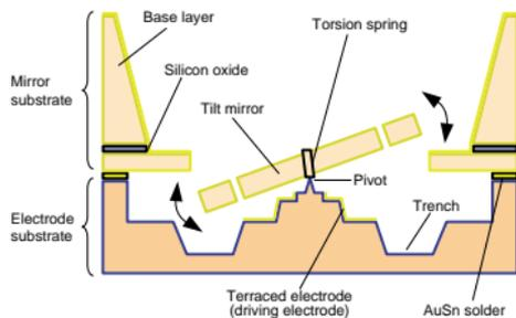
Fig. 2. Cross-sectional schematic of MEMS two-axis tilt mirror.
