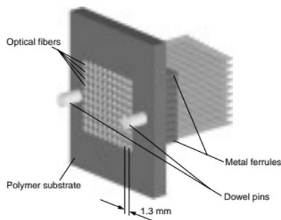
Fig. 4. Structure of 2D optical fiber array.
