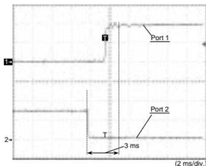
Fig. 8. Example of  $1 \times 2$  switching operation.
