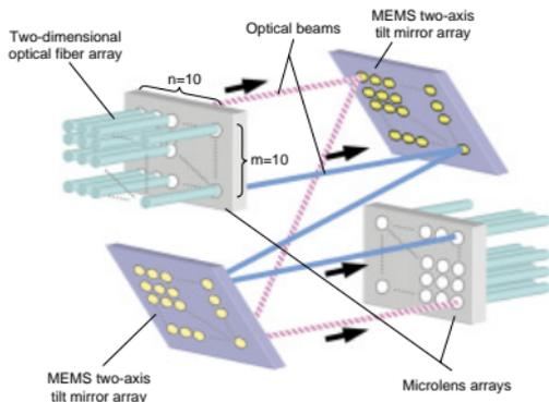
Fig. 1. Basic structure of 3D MEMS optical switch.
