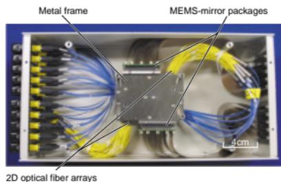
Fig. 5. Photograph of prototype optical switch module having 100 input and 100 output ports.
