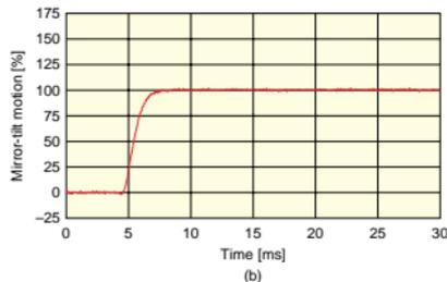
Fig. 7. Step response of MEMS-mirror motion (a) without and (b) with mirror-motion control.
