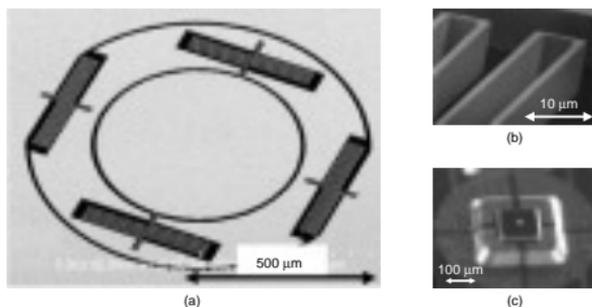
Fig. 3. (a) MEMS mirror, (b) the high-aspect torsion spring, and (c) 3D terrace electrode with a pivot.
