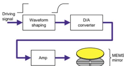
Fig. 6. Block diagram of mirror-motion controller.
