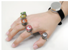
Fig. 2. Fulltime-wear text input mechanism (FingerRing).
