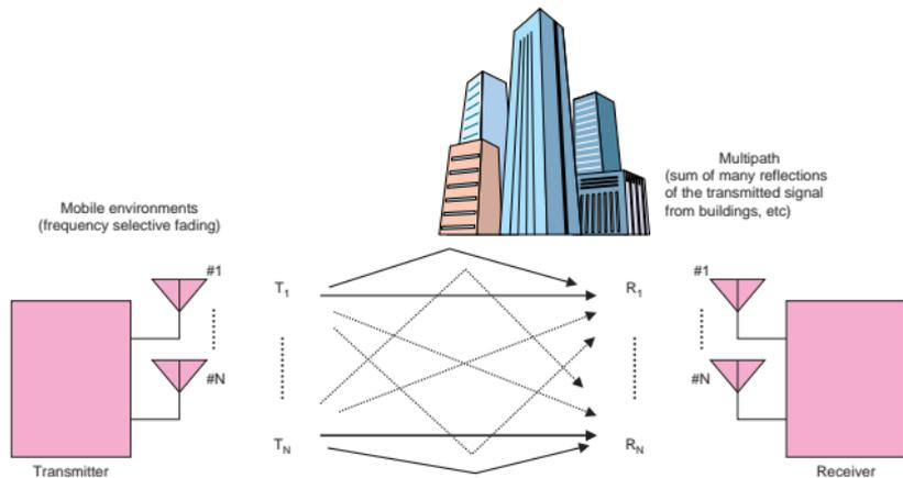
Fig. 1. Structure of SDM scheme.
