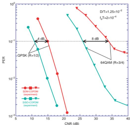
Fig. 8. PER performances of the SDM-COFDM prototype.
