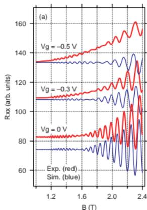
Fig. 2(a). Gate voltage dependence of SdH oscillations. Beating patterns in the SdH oscillations appear due to a spin-orbit interaction. By comparing the oscillations with the numerical simulation based on Rashba spin-orbit interaction, we can obtain spin-orbit interaction parameter  $\alpha$ .
