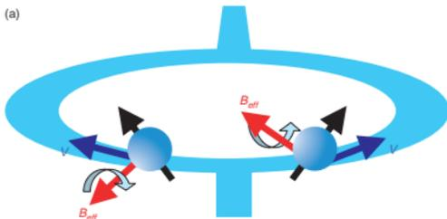
Fig. 3(a). Schematic of the spin-interference device. The electron spin feels an effective magnetic field perpendicular to its velocity direction; therefore, the precession angles of the left and right branches are different. A ring made of an InGaAs/InAlAs heterostructure is covered with a gate electrode, which controls the spin-orbit interaction.
