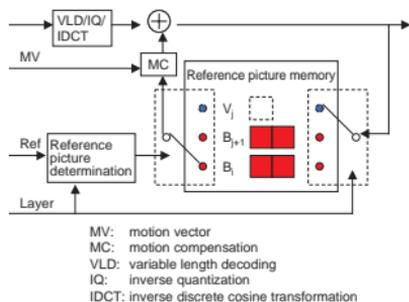
Fig. 7. Decoder configuration of HRPS.
