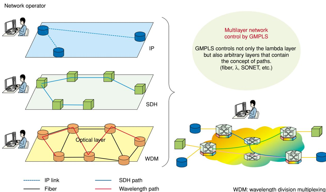
Fig. 1. Concept of multilayer network control.
