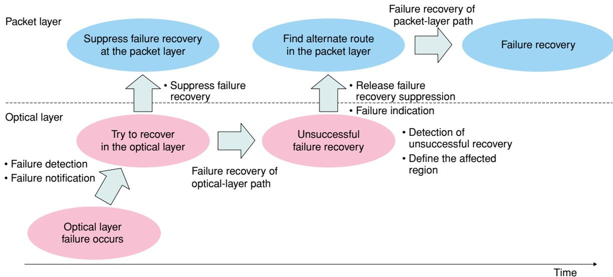
Fig. 3. Failure recovery through multilayer coordination.
