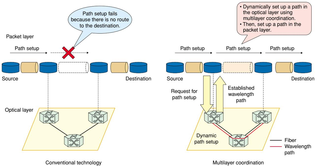
Fig. 2. Dynamic path control achieved by multilayer coordination function.
