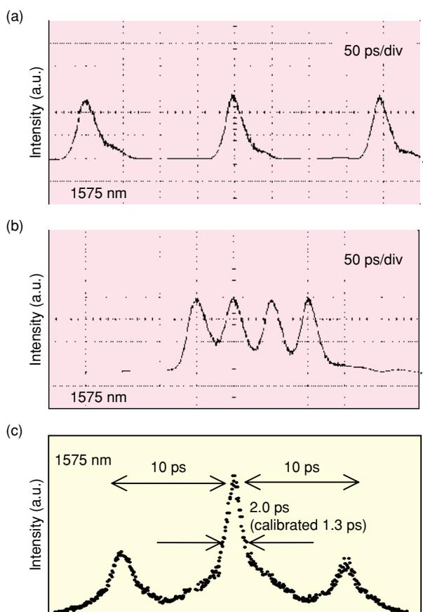
Fig. 13. Converted OTDM signals generated from 4 WDM signals. Time separation is (a) 200 ps (5 Gbit/s), (b) 50 ps (20 Gbit/s), and (c) 10 ps (100 Gbit/s).
