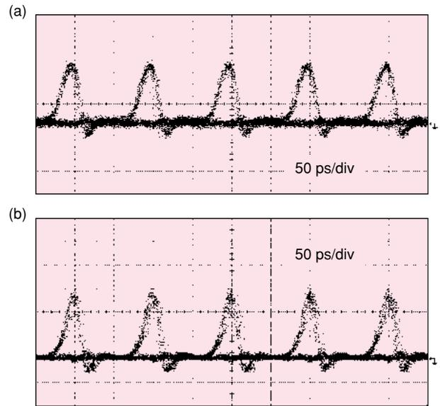
Fig. 8. Eye-diagrams of the demultiplexed signals measured after 1st processor. (a) Channel 1: 1561 nm and (b) channel 2: 1563 nm.
