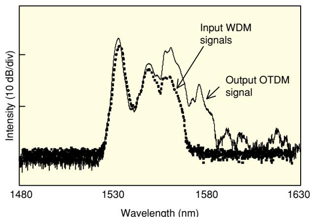
Fig. 12. Output spectrum of RS fiber for photonic conversion.
