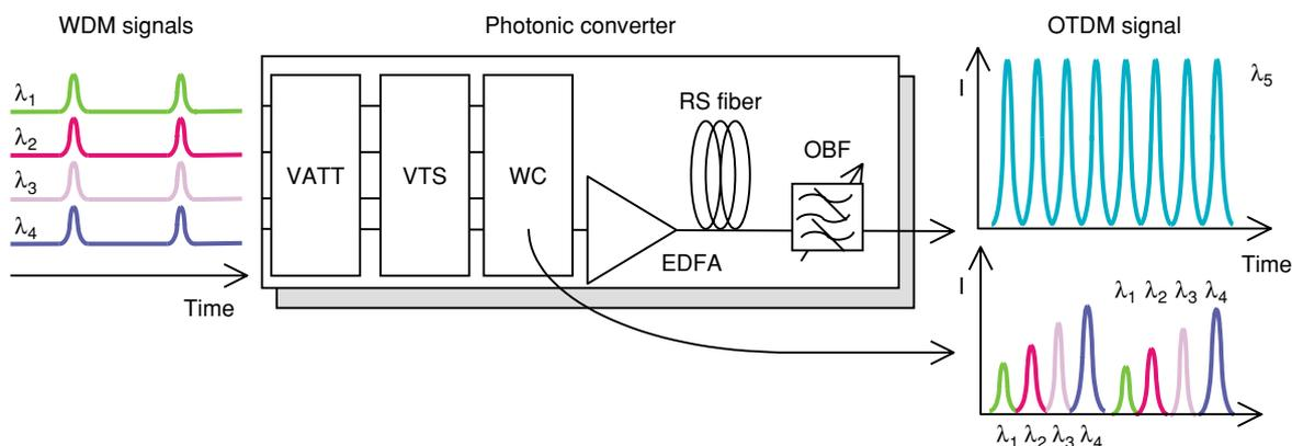
Fig. 2. Schematic configuration of photonic converter.
