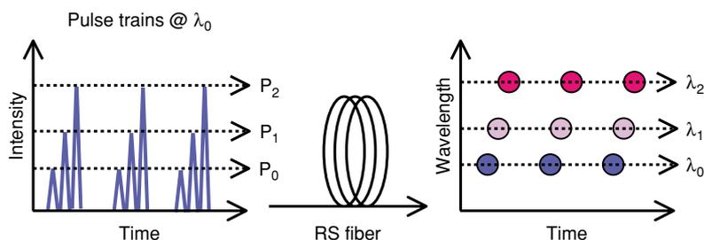
Fig. 1. Schematic concept of bit-by-bit self-signal recognition and simultaneous demultiplexing.
