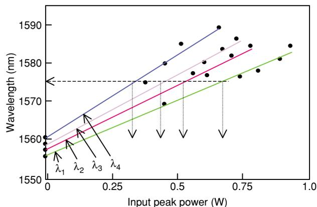
Fig. 6. Experimental dependence of the wavelength shift on input peak power.
