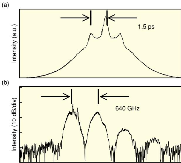
Fig. 7. Overlapping signals with relative intensity difference of 3 dB in contended optical packets. (a) Autocorrelation trace measured after PLC multiplexer with relative delay time of 1.5 ps and (b) spectrum of the overlapping signals.
