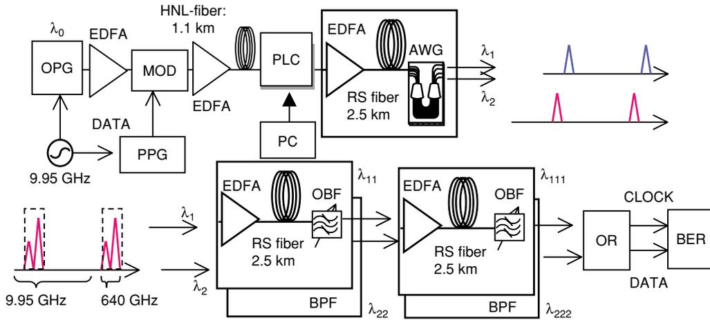
OPG: optical pulse generator, MOD: modulator, PPG: pulse pattern generator, PLC: PLC multiplexer, PC: personal computer, BPF: bandpass filter, OR: optical receiver, BER: bit error rate test set
