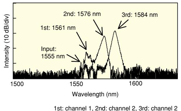
Fig. 10. Spectra of the demultiplexed signals measured after 2nd and 3rd signal processors.
