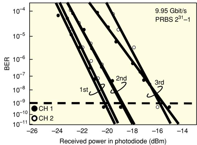
Fig. 9. BER performance measured after 1st, 2nd, and 3rd signal processors.
