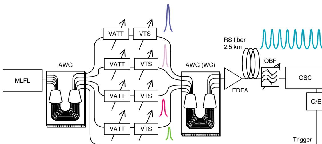
MLFL: mode-locked fiber laser, OSC: oscilloscope, O/E: optical-to-electrical converter
