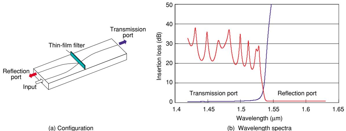
Fig. 4. Configuration and optical performance of WDM filter for video distribution.
