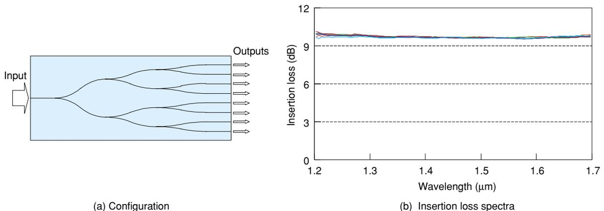
Fig. 2. Configuration and optical performance of  $1 \times 8$  PLC splitter.
