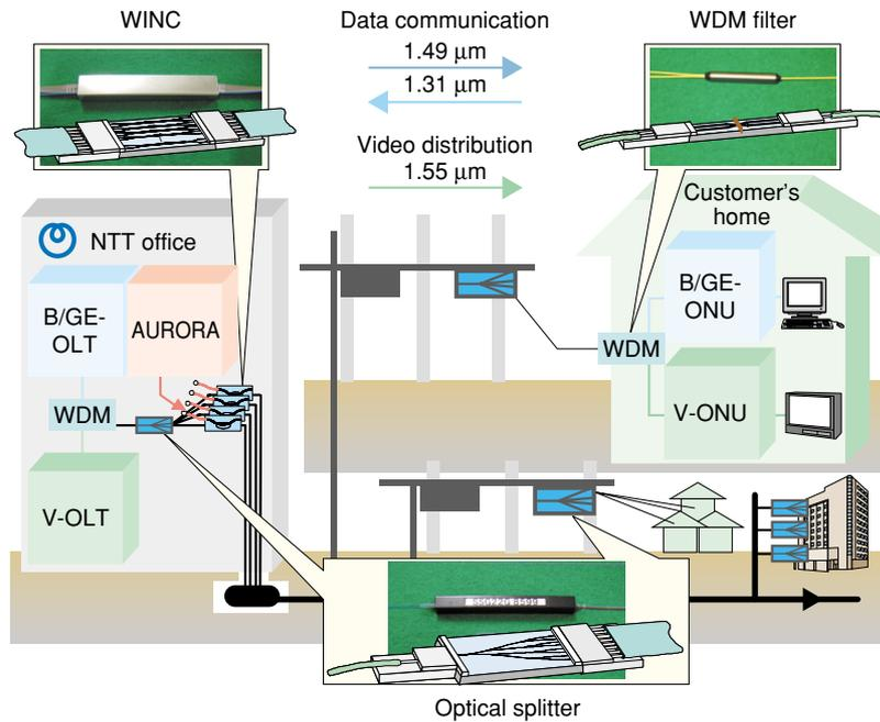
Fig. 1. Configuration of FTTH system.
