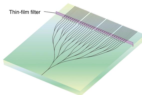
Fig. 5. Configuration of PLC splitter incorporating WDM function.
