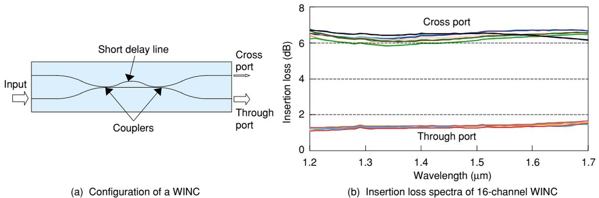
Fig. 3. Configuration and optical performance of 16-channel WINC.
