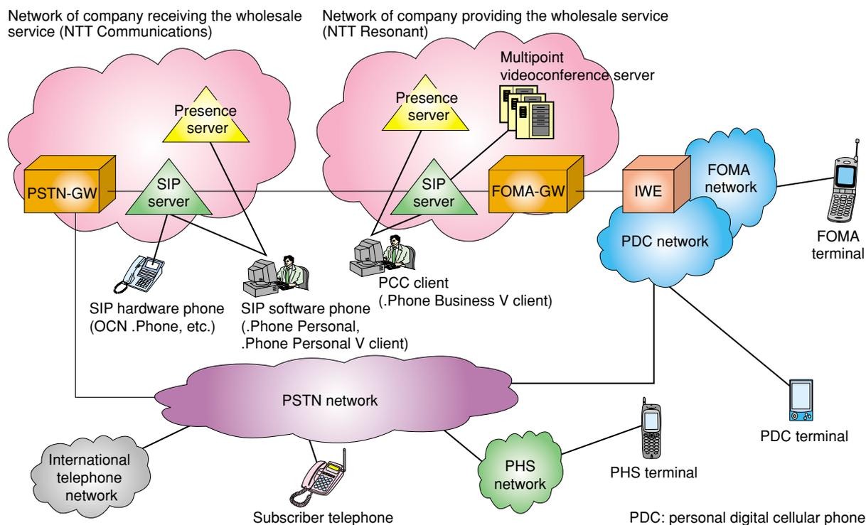
Fig. 1. PCC system and network configuration.
