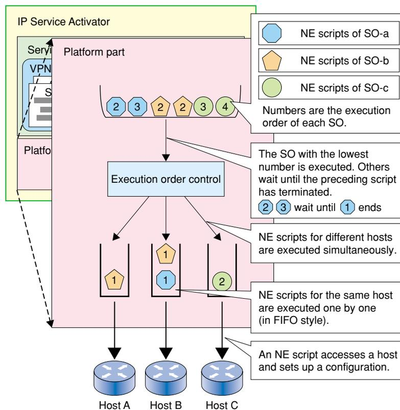
Fig. 4. Parallel execution and exclusive access control.
