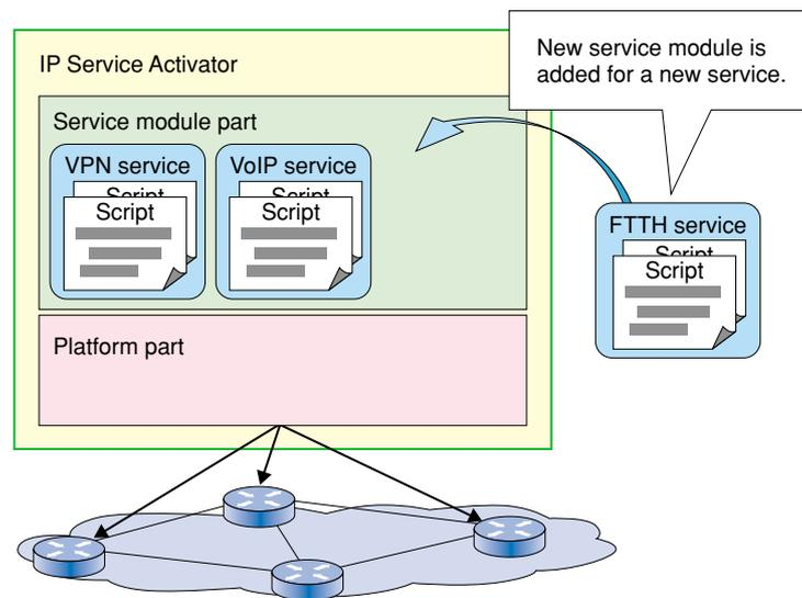
Fig. 2. System architecture of IP Service Activator.
