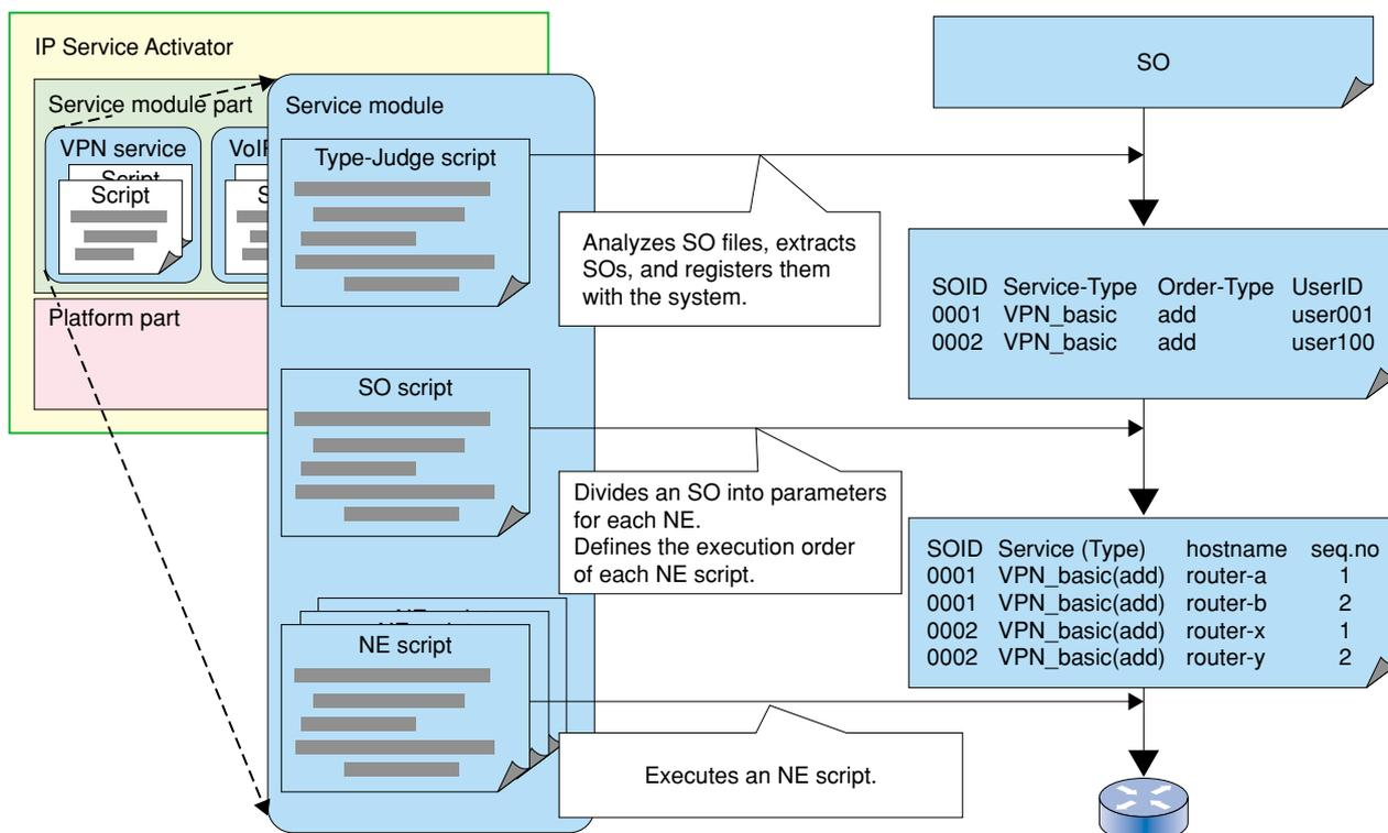
Fig. 3. Three scripts of a service module.
