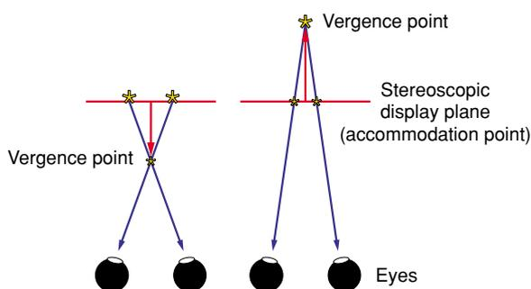
Fig. 1. Vergence point and lens accommodation with stereoscopic 3-D display.
