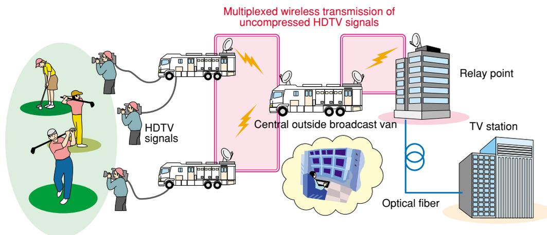
Fig. 1. Large-scale relay broadcast using ultrabroadband wireless communications.
