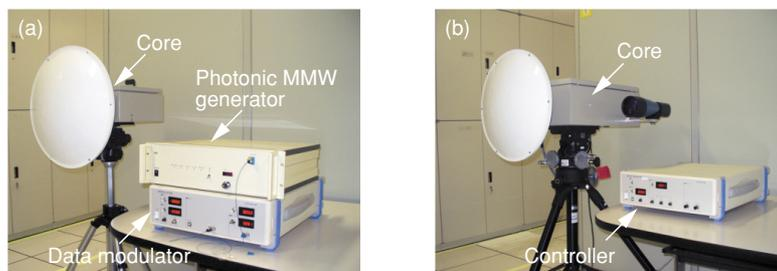
Fig. 3. Photographs of (a) transmitter and (b) receiver.
