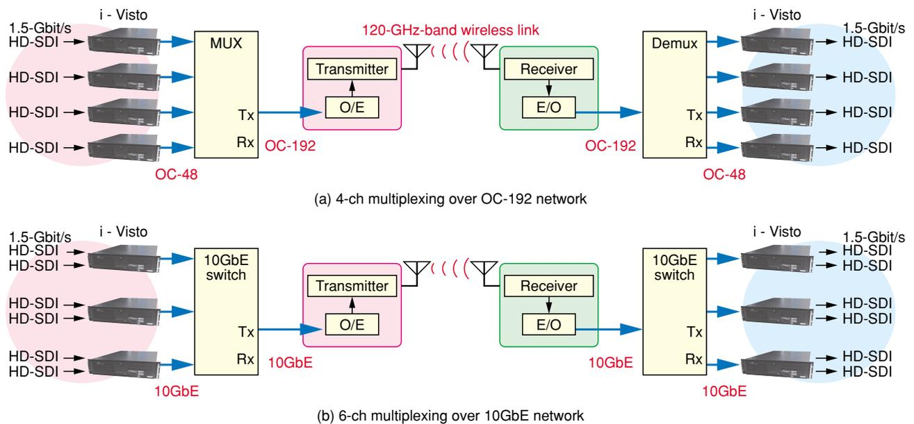
Fig. 4. Schematics of wireless links for multiplexed transmissions of uncompressed HD-SDI signals.
