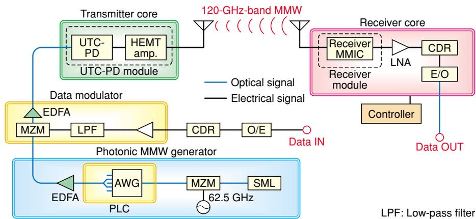
Fig. 2. Schematic of 120-GHz-band wireless link.
