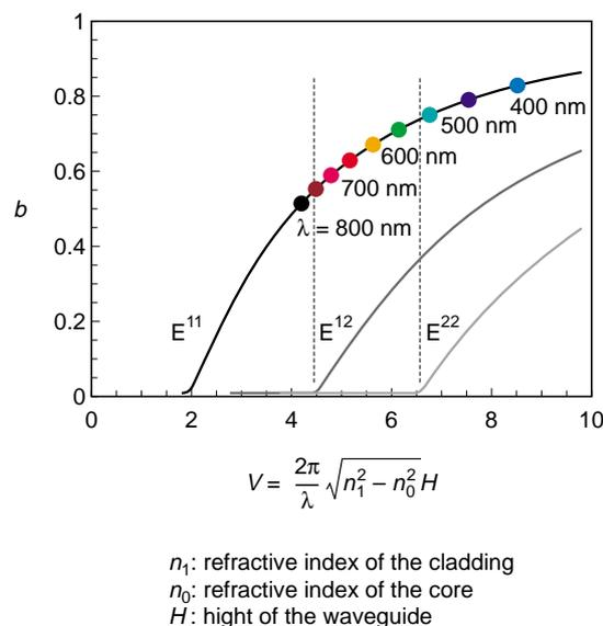
Fig. 2. Dispersion characteristics of silica-based waveguide for visible wavelength range.
