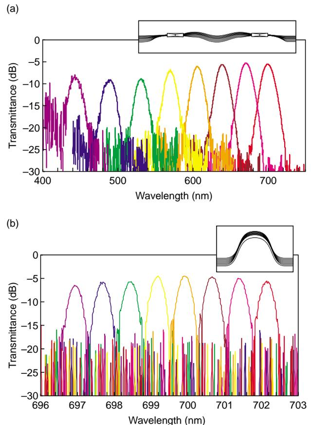
Fig. 5. Transmission spectra of (a) wide-range AWG and (b) narrowband AWG for visible wavelengths.
