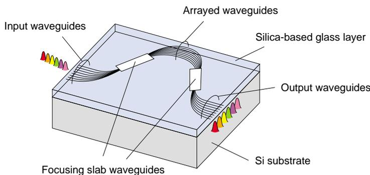
Fig. 1. Schematic configuration of silica-based arrayed-waveguide grating.
