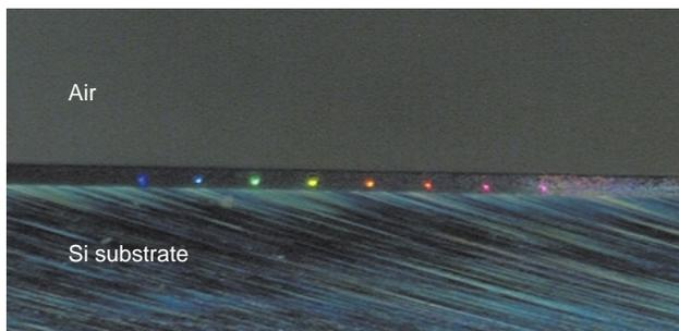
Fig. 4. Microscope image of eight outputs of wide-range AWG.
