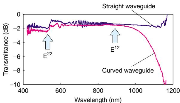
Fig. 3. Transmission spectra of straight and bent waveguides in the wavelength range from visible to near infrared.
