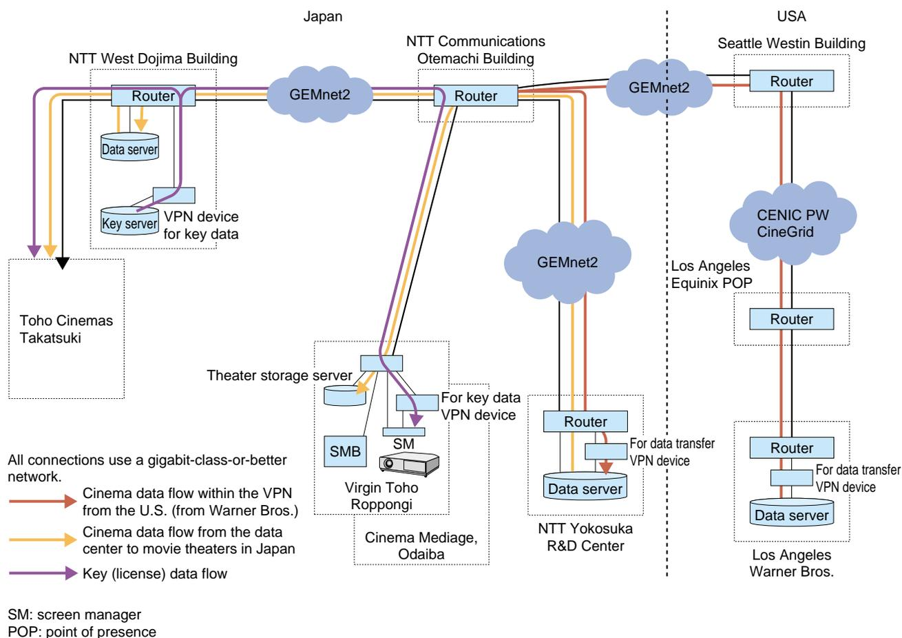
Fig. 3. Configuration of the trial system.
