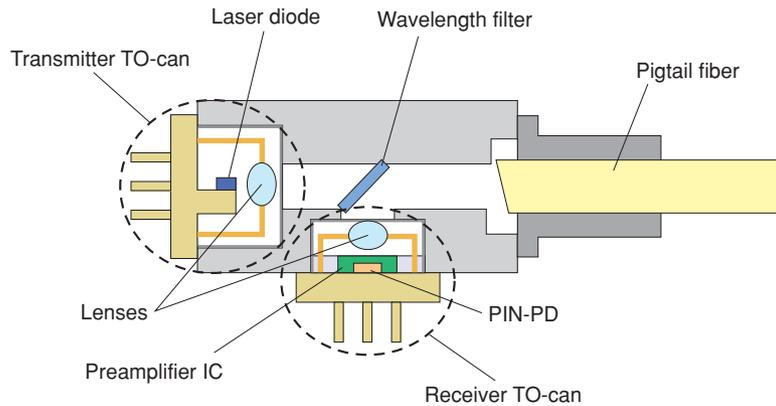
Fig. 2. Bi-directional optical transceiver.
