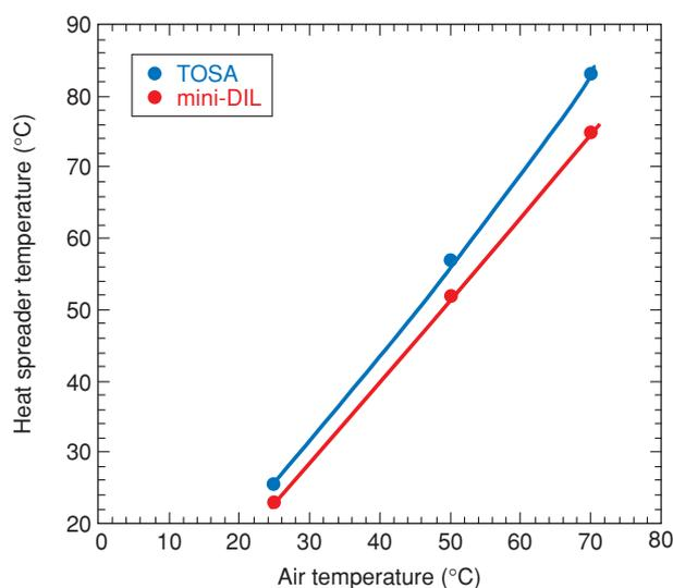
Fig. 2. Calculated heat spreader temperatures of TOSA and mini-DIL in XFP.
