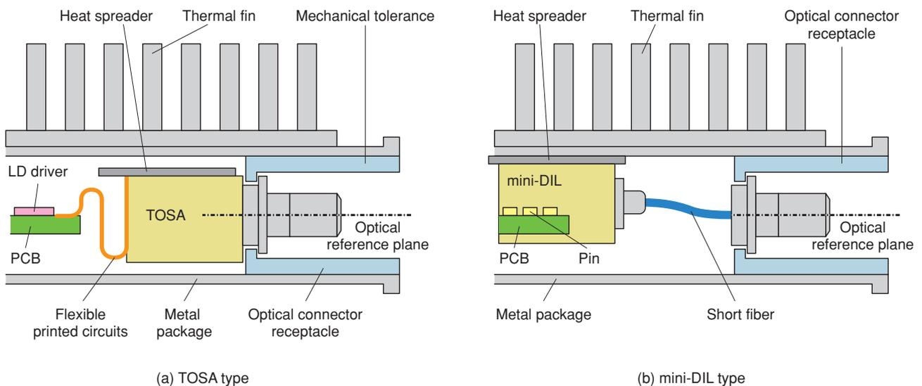
Fig. 1. Schematic outlines of the transmitter portions of XFPs.
