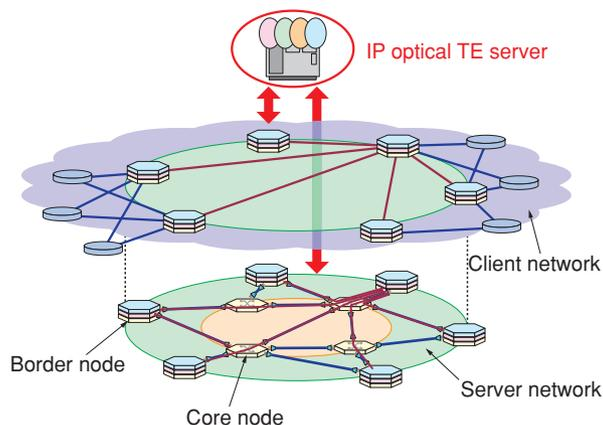
Fig. 1. IP optical multilayer network (MLN).
