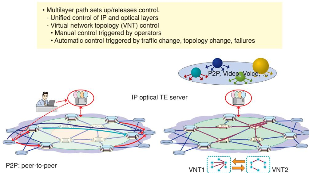
Fig. 2. IP optical multilayer traffic engineering.
