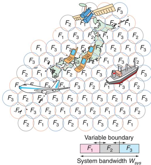
Fig. 1. Multibeam satellite communication system.
