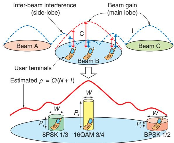
Fig. 6. Radio propagation within a beam.
