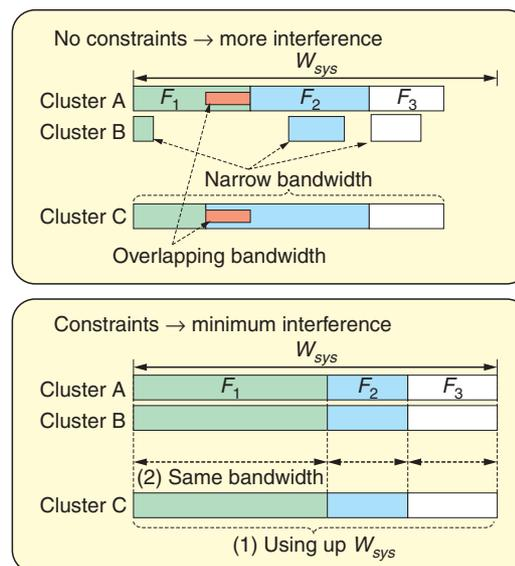
Fig. 4. Bandwidth constraints for the optimization algorithm.
