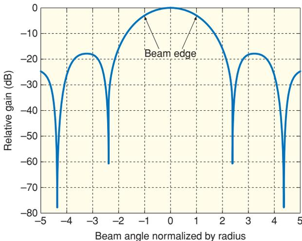
Fig. 2. Satellite antenna beam pattern.
