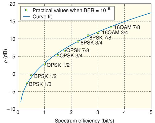
Fig. 3. Adaptive satellite modem performance.
