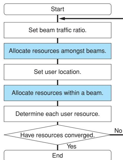
Fig. 8. Flow-chart of a two-layered resource allocation.
