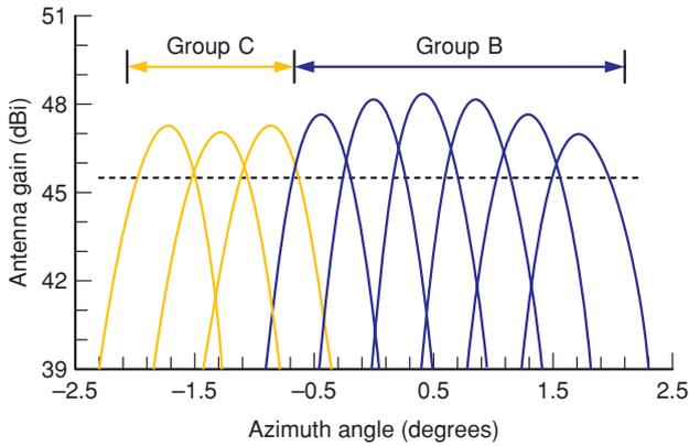
Fig. 9. Calculated antenna patterns for our feeder.
