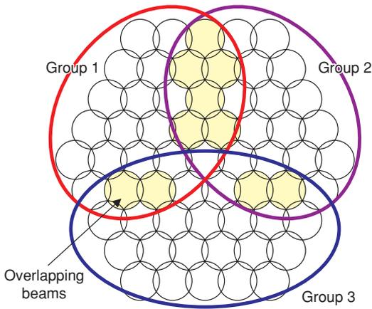
Fig. 5. Example of beam groups and overlapping beams.
