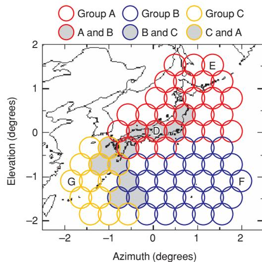
Fig. 8. Example of beam groups and overlapping beams.
