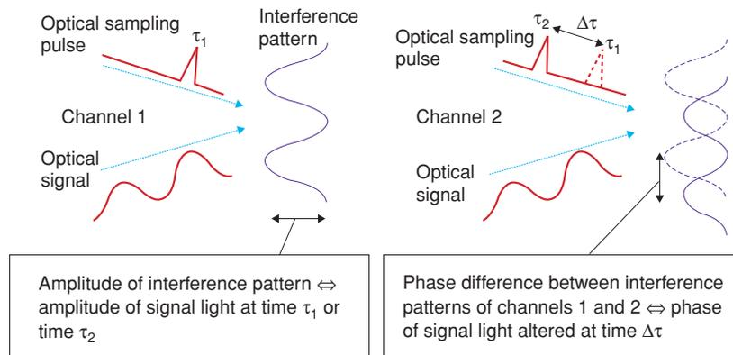
Fig. 1. Principle of linear optical sampling.
