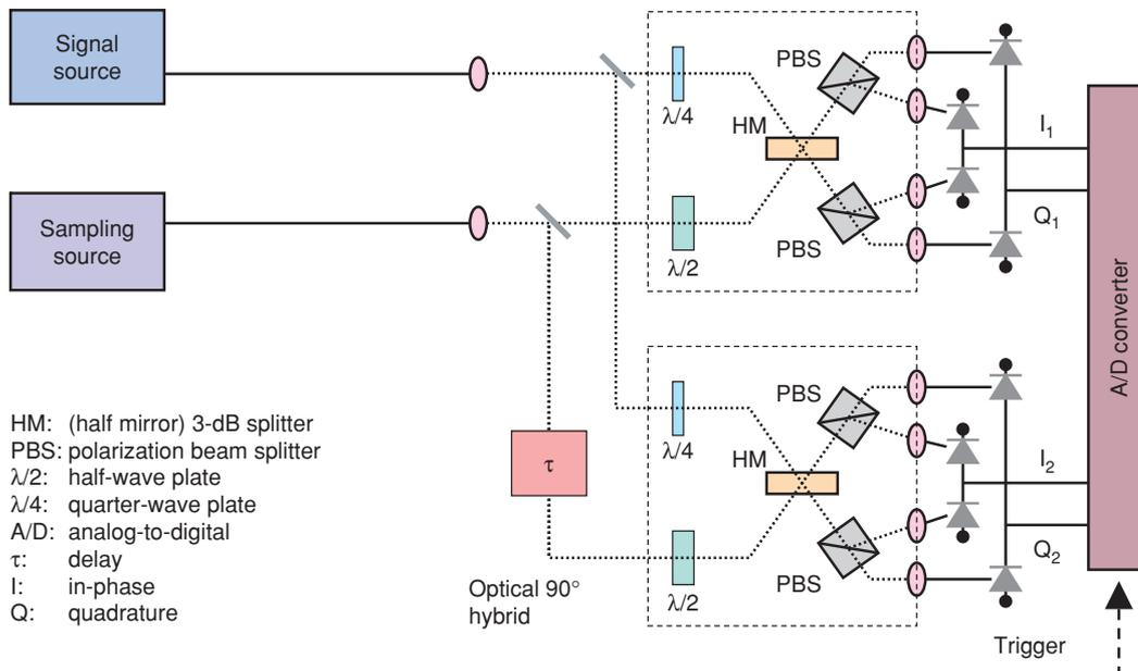
Fig. 2. Equipment configuration.
