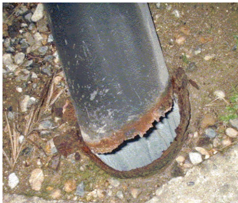
Photo 2. Collected pole 28 years after installation.
