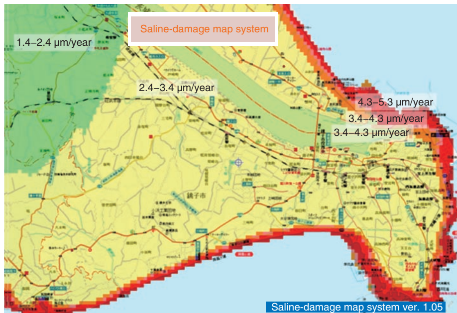
Fig. 10. Example of calculating zinc corrosion speeds by using the saline-damage map system (Choshi, Japan).
