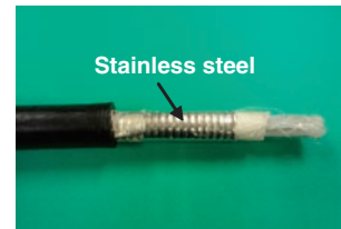
Fig. 13. Appearance of high-strength sheath cable.
