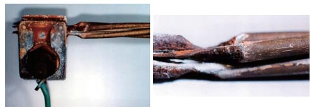
Fig. 5. Fractured AW messenger wire.
