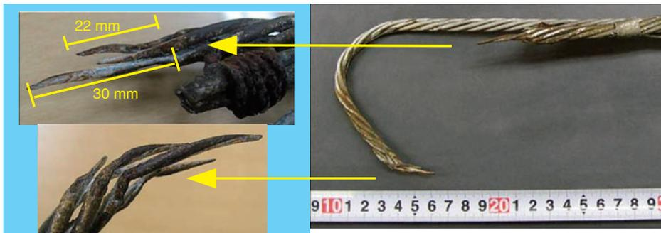
Fig. 1. Fractured aluminium corrosion-resistant wire grip.
